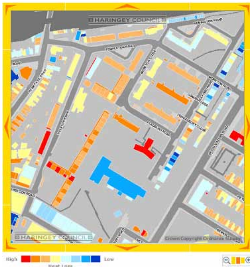
Figure 6: Heat loss maps showing areas within our project area in Haringey where high heat loss levels are most concentrated 12
